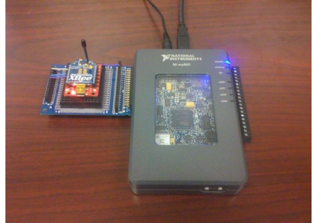
Fig. 11 myRIO connected to coordinator Xbee
